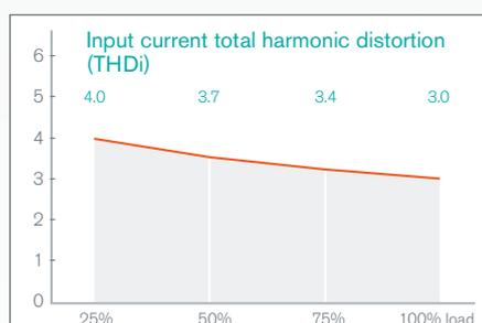
The outstanding low input current total harmonic distortion (THDi) helps to enhance the compatibility with generators. Low THDi eliminates possible interference with other equipment in the scheme, reduces the size of power cables, fuses and breakers at the input and avoids excess heating of power transformers.
