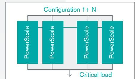
Up to 20 UPS units can be installed in parallel to achieve increased redundancy or more power.
