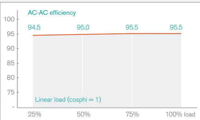
PowerScale exhibits state-of-the-art energy efficiency of up to 95.5%, therefore helping you to further reduce operating costs over the life of your UPS system. The flat efficiency curve is typical for all Newave products, and hence the fall in efficiency is marginal even at partial loads. This enables significant energy savings in every working condition.
