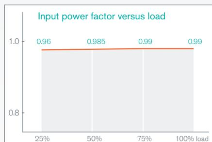
The input power factor of PowerScale is near unity. This is made possible by the advance booster PFC (Power Factor Correction) circuit of Newave's transformer-less technology. As a result there is no need for a filter for phase compensation. When using PowerScale, the UPS system respects the power grid regulations, and therefore achieves important energy savings.
