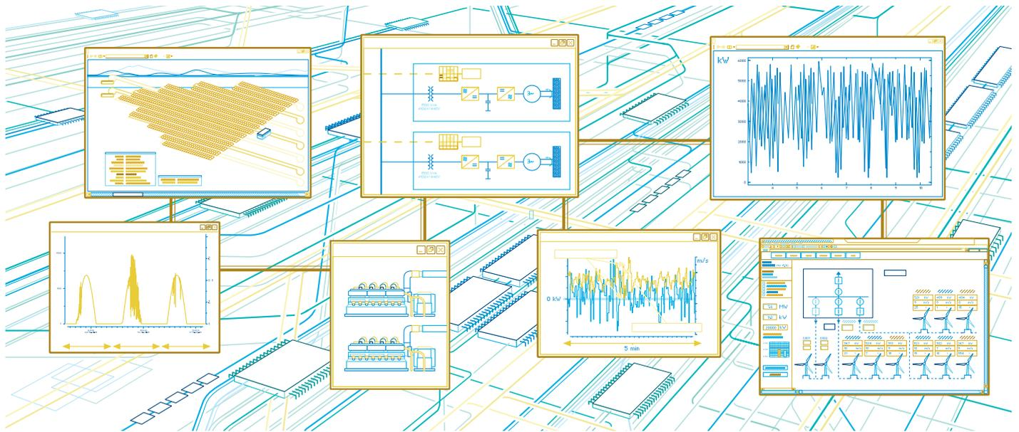
To control the generation and consumption of real and reactive power, the MGC600 consists of any configuration of IDC products. Some of the control and monitoring systems utilize a power measurement meter. This is used to verify how much real or reactive power is being generated or absorbed.
